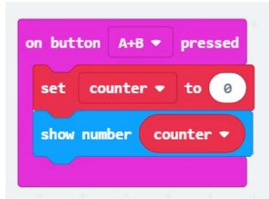
With the code now complete, click on download to download a HEX file to your Downloads folder, and then flash the code to your micro:bit by connecting the micro:bit to the computer, and dragging the HEX file to the micro:bit drive in your file manager. Once flashed, remove the micro:bit and power it from a USB battery or using the 2 x AAA battery holder that came with your micro:bit.
