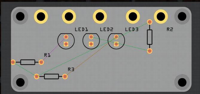
There are a few important things to note about PCBs before we start the layout of ours. The PCB we will be creating is a "Two-Layer Board" which means it has two sides in which you can have traces. It's good practice to put all the traces on the back of the PCB if possible so it looks nicer when produced. PCBs also have a layer called "Silkscreen" in which you can put text and images. They also have a "Soldermask" layer which is the colour of the PCB.
