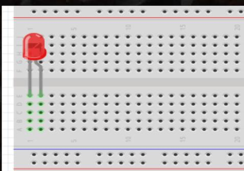
Our breadboard is split into two halves, each half has 5 rows. You'll see that there are "coordinates" on the breadboard to mark the holes. Drag the Red LED from the parts view into the top two holes of the bottom half like the image on the left. There we go! You've just dragged your first component onto the breadboard. Now, right click on the red LED and click duplicate. Skip two holes and on the same row drop the duplicated LED.
