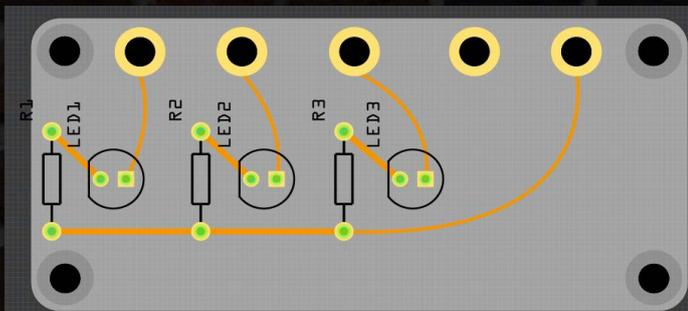
The last step of wiring up our PCB is to connect all the resistors to the GND pin of the micro:bit. Create traces between each bottom connector of the resistors and the wire the one on the right to the last pin on the micro:bit as shown below. Once that is complete you have finished routing your PCB!
