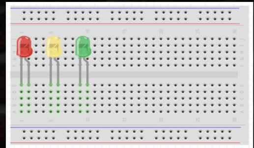
There we have it, our LEDs are now in place. The next thing we need to do is add some resistors. Scroll to the top of the CORE category and you'll find a resistor icon. Drag and drop it underneath the breadboard.
