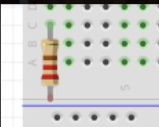
Next, what we need to do is rotate the resistor so that it's vertical rather than horizontal. Select the resistor and at the bottom of the Fritzing window, you'll see a rotate button. Click it once to rotate the resistor so that it's vertical. Now once you've done that, drag the resistor so that the top leg is in the second hole underneath the short leg of the Red LED
