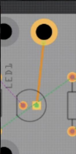
Now we have the PCB layout done, it's time to create some traces! Each screw hole on our template has a small connector. If you zoom in on a screw hole you'll be able to see it. Each component also has holes in which the components legs will go through, we can use these connectors to draw a trace from the micro:bit to the component.
