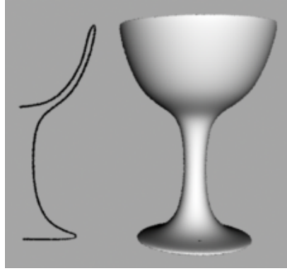
Figure 17: Revolve Object (left: Curve, right: Surface of Revolution)
