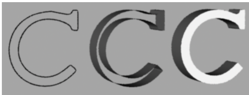
Figure 18: Extrude Object (left: Curve, middle: normal Extrusion, right: Extrusion with Caps)
